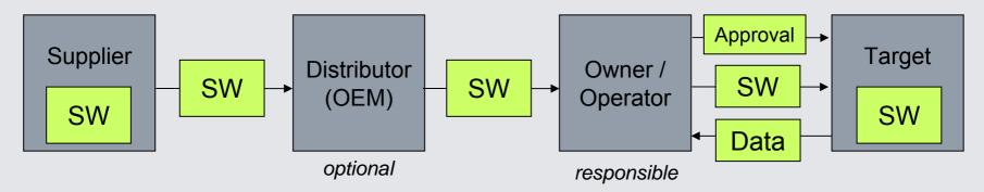
*More general:* IT system with networked devices in the field performing safety-critical and/or security-critical tasks. Field devices require secure update of embedded software.
