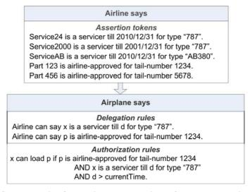
Fig. 4 SecPAL policy for an airplane accepting software part loading
