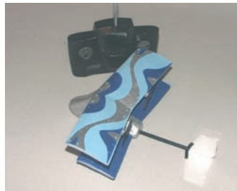
Two-channel control operates the 'throttle', speed controller and differential power to the twin motors for directional control, they are fully proportional. The minuscule aerial can be seen projecting out of the tail boom, range is perfectly adequate.
